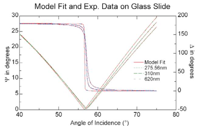
Figure 3. Accurate measurement of variable angle ellipsometric data near the Brewster angle on a glass microscope slide, using VASE with AutoRetarder. This very accurate measurement of  $\Delta$  would not be possible with a standard RAE or RPE system.
