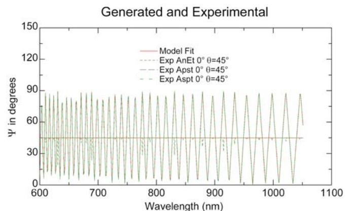
Figure 5: G-VASE™ data acquired on LiNb substrate. The oscillations in the data are due to a conversion of p-polarized light to s-polarized and vice versa. Six data points are acquired at each wavelength when performing a G-VASE™ measurement.
