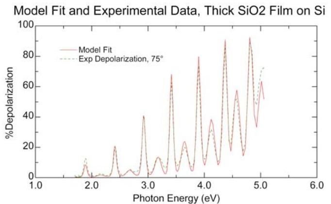
Figure 4a and 4b. Spectroscopic ellipsometric (a) and depolarization (b) data acquired on a 10540Å SiO<sub>2</sub> film on Si by a M-2000. To fit the depolarization data, a spectrometer bandwidth of 7nm (assuming a Gaussian profile) and a film thickness non-uniformity of 0.44% were included in the optical model
