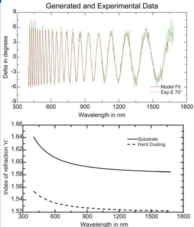
Figure 2a and 2b. Ellipsometric  $\Psi$  (not shown) and  $\Delta$  (a) data acquired with a retarder-equipped RAE system<sup>5</sup> on a polycarbonate lens with a thick (4.35mm) hard coating. Accurate measurement of the period and amplitude of oscillations in both  $\Psi$  and  $\Delta$  (notice it is very close to zero) enabled accurate determination of the film thickness and optical constants (b).
