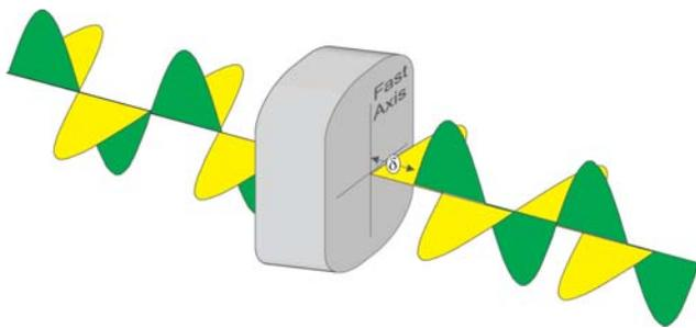
Figure 1. Retarder element introducing a phase shift between the two light constituents.
